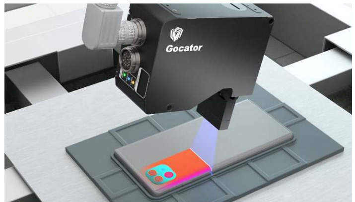
Gocator® 2522 scanning cell phone cover glass assembly
